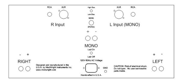
Caution: Do not connect the Mono binding post to any speaker circuitry that grounds any speaker lead. If either terminal of the Mono binding post are connected to GROUND when operating in bridge-mono mode, damage to the amp may occur. It is not recommended to run the amplifier in bridged mono into 20hm loads.
