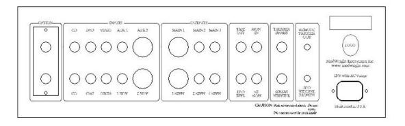
HT/BP input is meant for integrating 2CH into a Multi-Channel or Home Theater system. When used in this mode, home theater preamp or processor is connected to HT/BP inputs and signal is output straight to 2CH main stereo outs. This allows direct connection to front L/R channel amp(s) with no sonic impact from LS 100 preamp.
